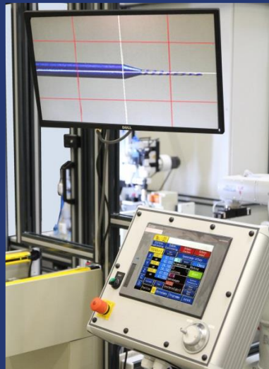
Monitor and Touch screen-operators terminal for process surveillance and control
