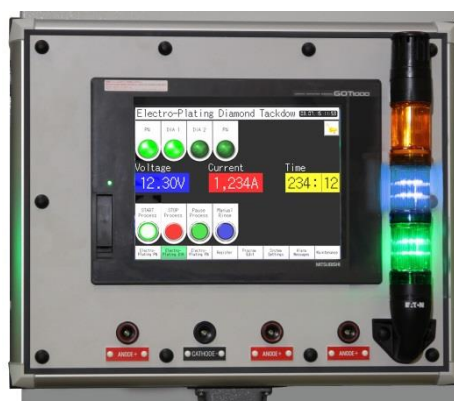
3-stage automatic process-run control and preset of the electro-plating parameters by the Touch screen operators' terminal (DBS XXA-45 control).
