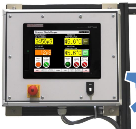
Pre-set and monitoring of the process and bath parameters by means of the Touch screen operator terminal (PBS-845/001 control)
