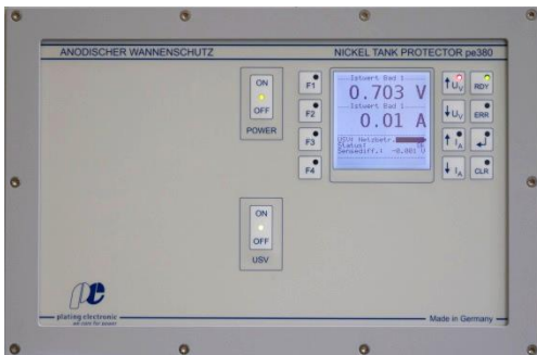
Operation panel for anodic tank protection (Protectostat) Nickel regulator for monitoring and stabilization of plating bath
