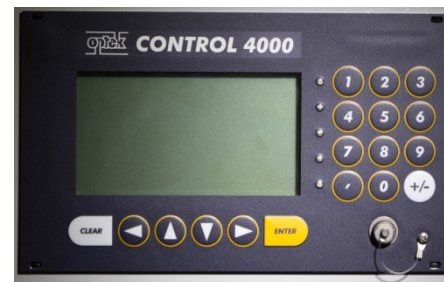
Operation panel for anodic tank protection (Protectostat) Nickel regulator for monitoring and stabilization of plating bath
