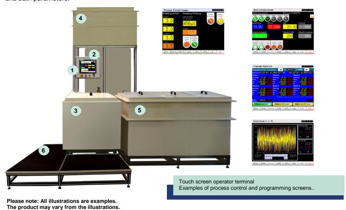
Touch screen operator terminal for process control, programming, pre-set and monitoring of:
