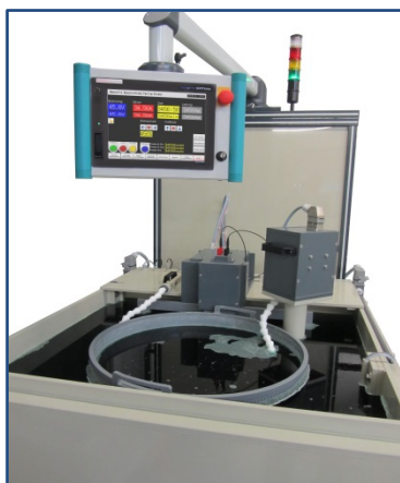
Electro-plating station of the DBE-1/100x120x80 with electro-plating cassette, rotation unit, lifting/lowering installation and Touchscreen operators' terminal
