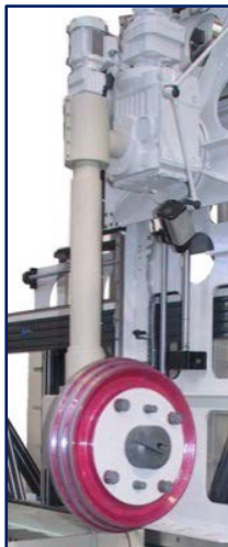
Grinding wheel mounted to swivel and rotation unit
