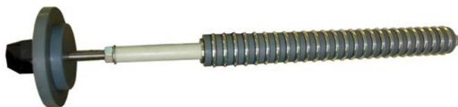
Holding fixture for the etching of dicing blades with AL-hub for 27 pcs each; assembled (left); components (right)
