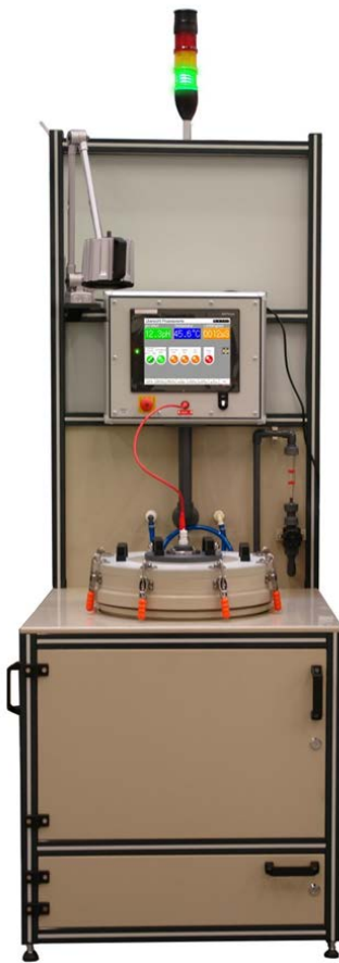
Rotational reverse-plating unit RBE - 1 rotational plating vessel with lid - Flow meter and diaphragm valve for electrolyte flow regulation - Rotation max. 500 rpm - 1 rotational reverse-plating control RBS 10A-45/001
