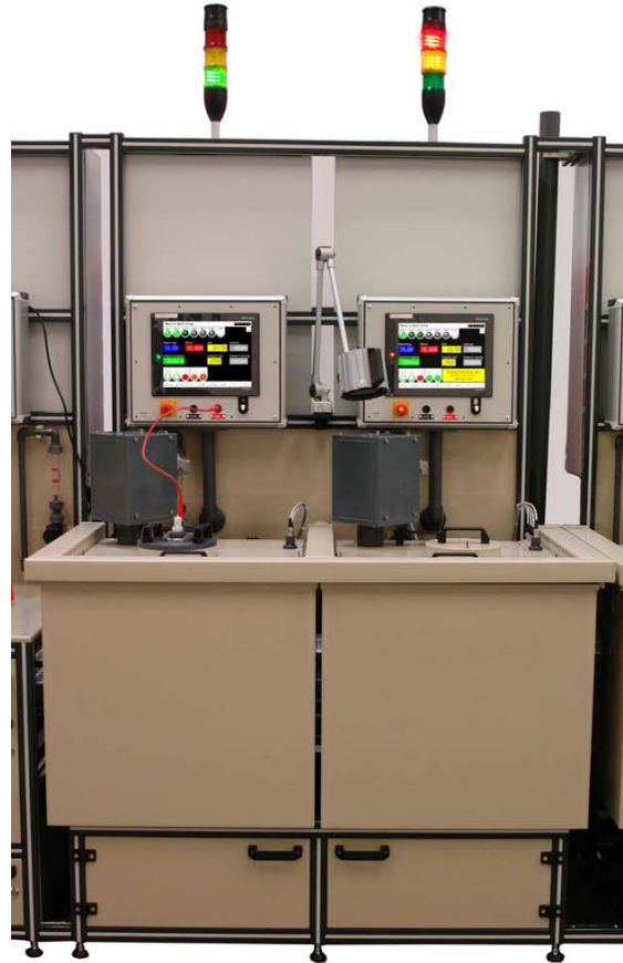
Thick-nickel plating unit DVE 2/56-56-50/001 - 2 electro-plating tanks with rim exhaustion - 2 horizontal rotation units - 2 thick-nickel plating controls DVS 10A-45/001 with built-in motor control
