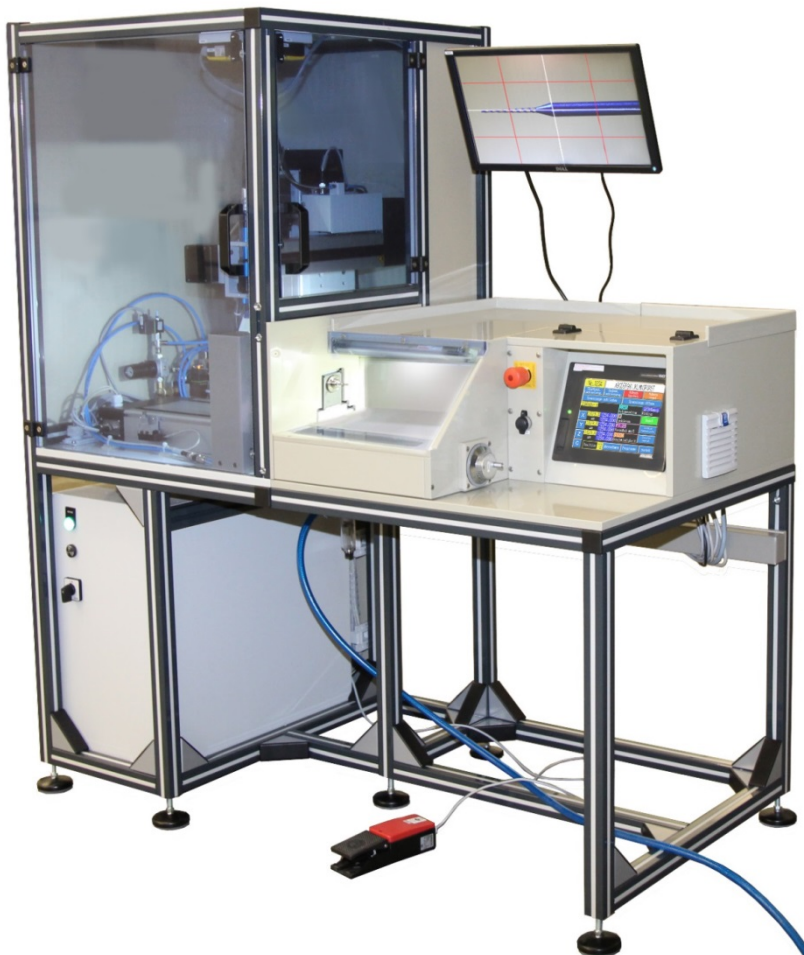
Varnishing unit with three-axes linear guide and volumetric paint dosing
