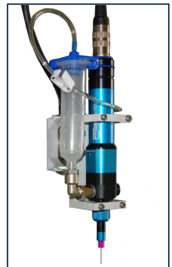
Volumetric varnish dosing system
