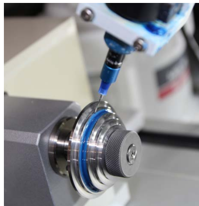
Masking varnishing of a grinding wheel blank. Free positioning of the paint dispenser allows masking work pieces with complex shapes and undercuts.
