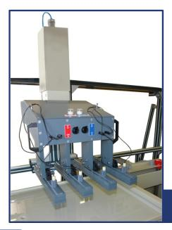
Transport carriage with lifting and lowering installation with four contact fixtures in place
