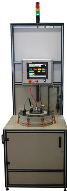
Rotational reverse-plating unit RBE 1/45-49/001 - 1 rotational plating vessel with lid - Flow meter and diaphragm valve for electrolyte flow regulation - Rotation max. 500 rpm - 1 rotational reverse-plating control RBS 10A-45/001
