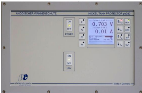
Operation panel for anodic tank protection (Protectostat)
