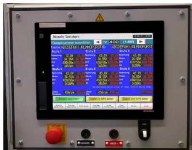
Touchscreen operator terminal of the PRS (Electrolyte constancy) Display examples of bath parameters, temperature recording, Temperature setting, AH-counter.
