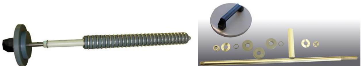
Holding fixture for the etching of dicing blades with AL-hub for 27 pcs each; assembled (left); components (right)
