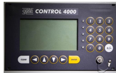
Nickel regulator for monitoring and stabilization of plating bath
