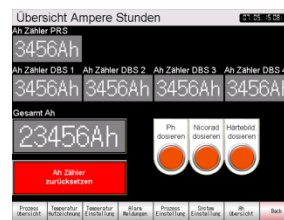
Touchscreen operator terminal of the PRS (Electrolyte constancy) Display examples of bath parameters, temperature recording, Temperature setting, AH-counter.
