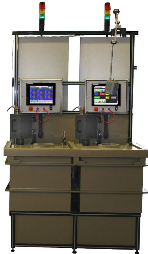
Thick-nickel plating unit DVE 2/56-56-50/001 - 2 electro-plating tanks with rim exhaustion - 2 horizontal rotation units - 2 thick-nickel plating controls DVS 10A-45/001 with built-in motor control
