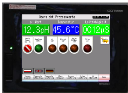
Adjustment and monitoring of the bath parameters by the Touch screen operators' terminal (PRS control)
