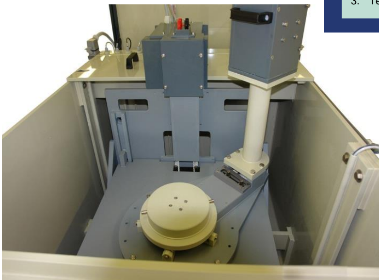
Lifting/lowering table with mounted rotation unit and bayonet catch fitted into electro-plating tank.
