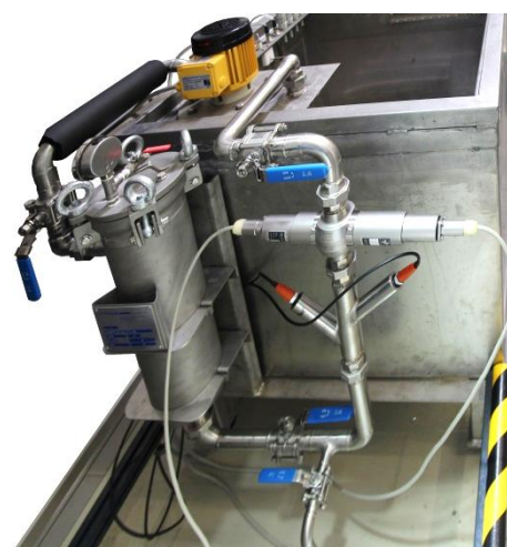
袋式过滤装置和监测镀槽的传感器 Filter bag unit and sensors for monitoring the plating bath
