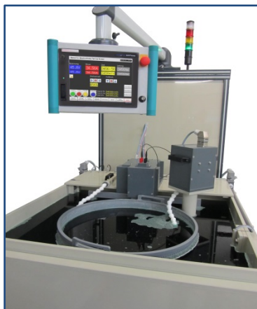
DBE-1/100x120x80 电镀站带有电镀箱， 旋转装置，升降装置，以及终端操作触摸 屏 Electro-plating station of the DBE- 1/100x120x80 with electro-plating cassette, rotation unit, lifting/lowering installation and Touchscreen operators' terminal
