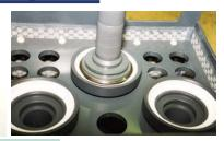
活塞环磨轮的装置系统 Fixture system for piston-ring grinding wheels
