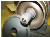
大磨轮和磨辊的夹具系统 Fixture system for large grinding wheels and grinding drums
