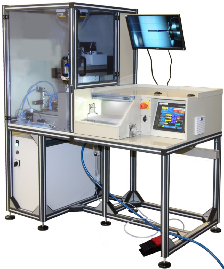
带有三轴导轨的上漆装置以及根据压力加药的上漆系统 Varnishing unit with three-axes guide and pressure based varnish dosing system
