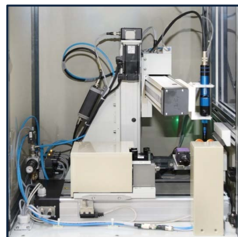
带有 3 轴导轨与容积配量系统的上漆装置 Varnishing unit with three-axes linear guide and volumetric paint dosing
