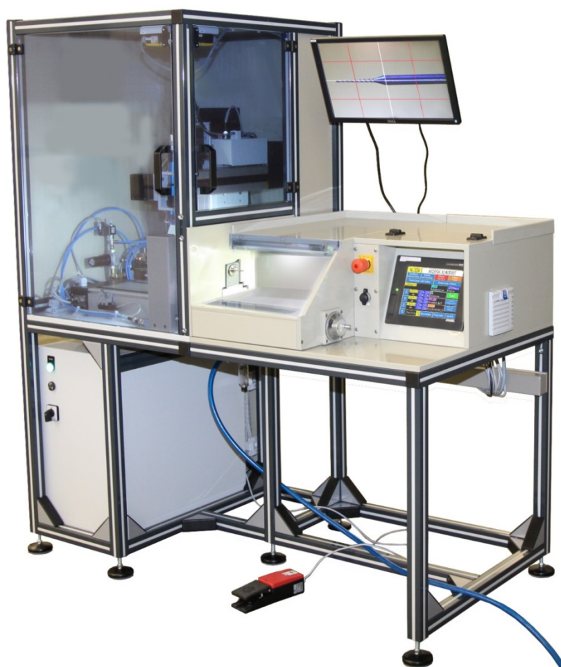
带有 3 轴导轨与容积配量系统的上漆装置 Varnishing unit with three-axes linear guide and volumetric paint dosing
