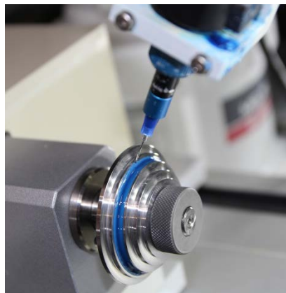
磨轮毛坯的绝缘漆 Masking varnishing of a grinding wheel blank. 上漆装置的自由定位功能可以为带有凹槽的复杂形状工件上漆 Free positioning of the paint dispenser allows masking work pieces with complex shapes and undercuts.
