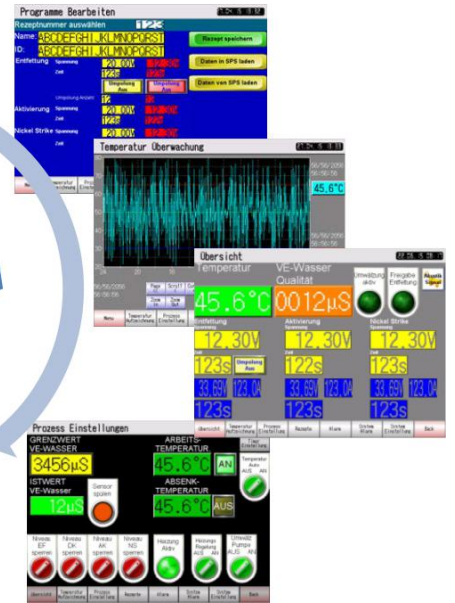
Pre-set and monitoring of the process and bath parameters by means of the Touch screen operator terminal (PBS-845/001 control) 通過終端操作觸摸屏預設和監控處理及槽參數 (PBS-845/001)
