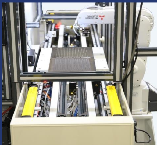
6-station linear transport unit for holding pallets 装托盘的 6 站式线性运输单元
