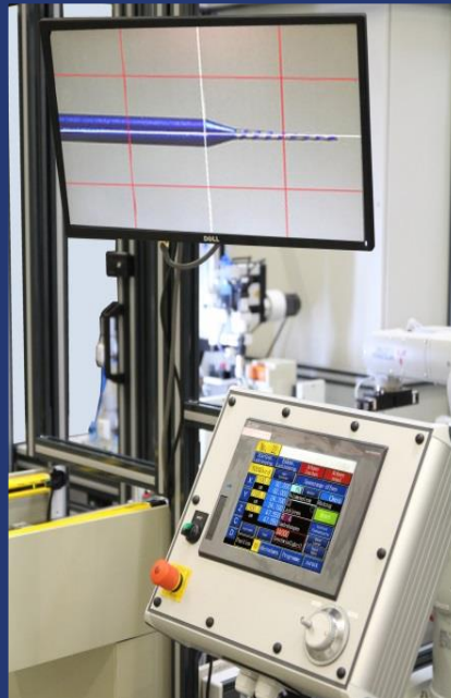
Monitor and Touchscreen-operators terminal for process surveillance and control 用于过程监视与控制的监视器与触屏操作终端
