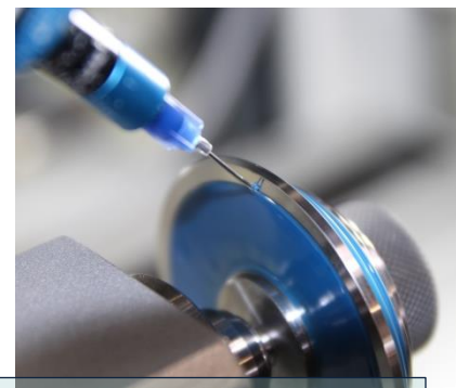
磨轮毛坯的绝缘漆 Masking varnishing of a grinding wheel blank.
