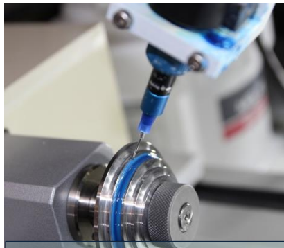
磨轮毛坯的绝缘漆 Masking varnishing of a grinding wheel blank.
