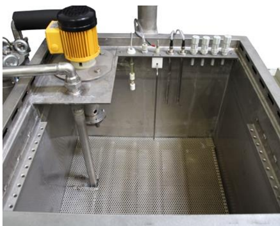
镀槽的内视图 Inside view of plating tank
