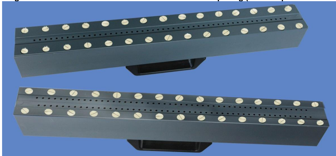
Single and double-row contact fixtures for nickel electro-plating (bath temperature max. 60 °C)
