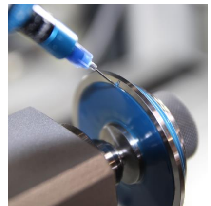
磨轮毛坯的绝缘漆 Masking varnishing of a grinding wheel blank. 上漆装置的自由定位功能可以为带有凹槽的复杂形状工件上漆 Free positioning of the paint dispenser allows masking work pieces with complex shapes and undercuts.
