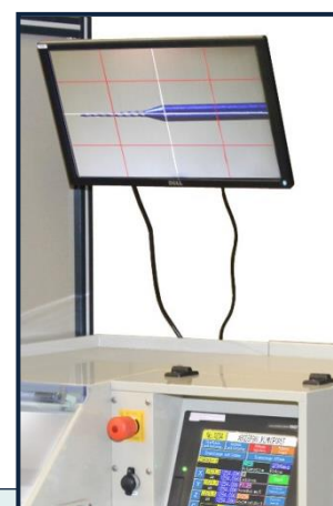
用于监控上漆的显示屏 Monitor to check varnishing
