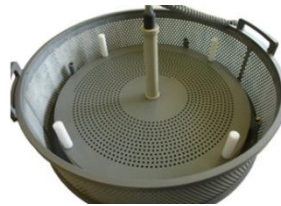
带有钛阳极篮（图中不可见）的接触夹具和屏蔽盘安装在电镀盒里 Contact fixture with titanium anode baskets (not shown) and shielding disc mounted into electro-plating cassette
