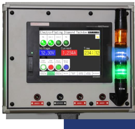
通过终端操作触摸屏调控 3 阶段自动程序操作和预设电镀参数(DBS XXA-45 调控) 3-stage automatic process-run control and preset of the electro-plating parameters by the Touch screen operators' terminal
