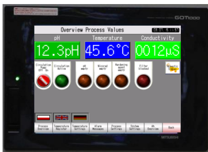
通过终端操作 触摸屏设置和监控槽参数 (PRS 调控) Adjustment and monitoring of the bath parameters by the Touch screen operators' terminal (PRS control)
