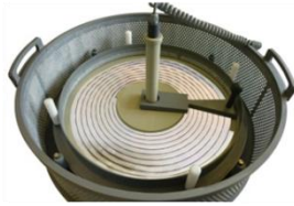
带有耙子的接触夹具平整金刚石砂粒 Contact fixture with rake to equalise diamond grits distribution
