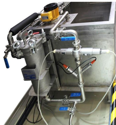
袋式过滤装置和监测镀槽的传感器 Filter bag unit and sensors for monitoring the plating bath
