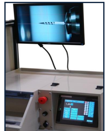
用于监控上漆的显示屏 Monitor to check varnishing
